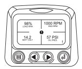
Indicates Auxiliary Gage Fault
